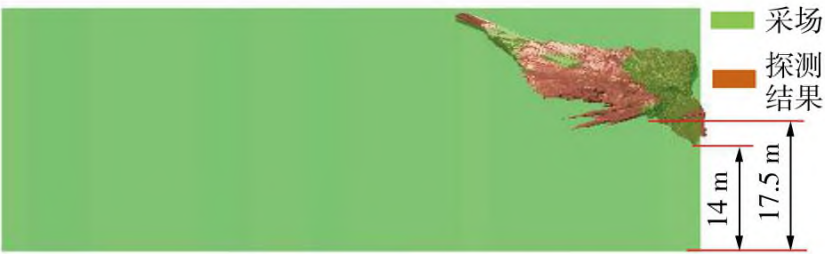
图2 7635采场的冒落情况 Fig. 2 Results of roof caving in 7635 stope
