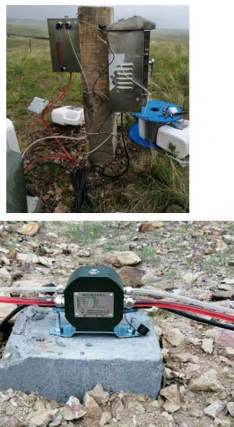
图6 静力水准仪布设 Fig. 6 Layout of static level
